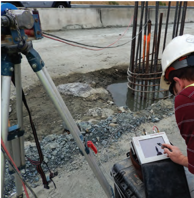
Shaft cross section with four tubes, six paths are tested.
