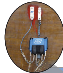
Smart accelerometer and strain transducer, offshore version.
