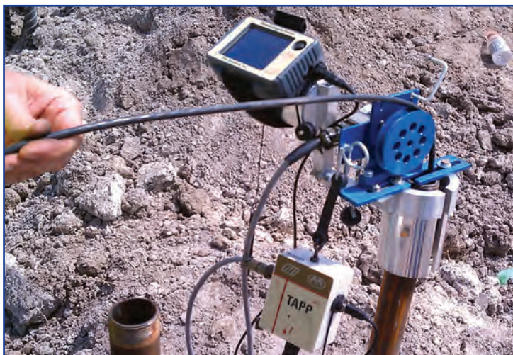
Thermal Integrity Profiler (Probe System).
